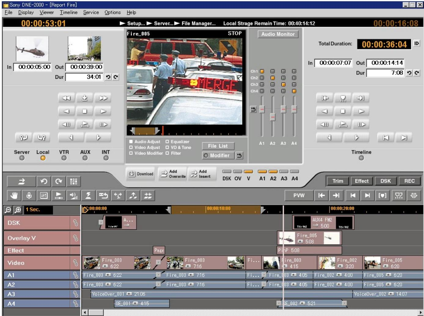
The GUI of the DNE-2000 comprise four main sections (from top left to bottom)
