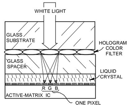
Figure 11. Hologram color filter schematic for SD-ILA device
