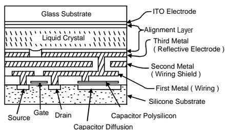
Fig. 4. Cross-section of D-ILA device
