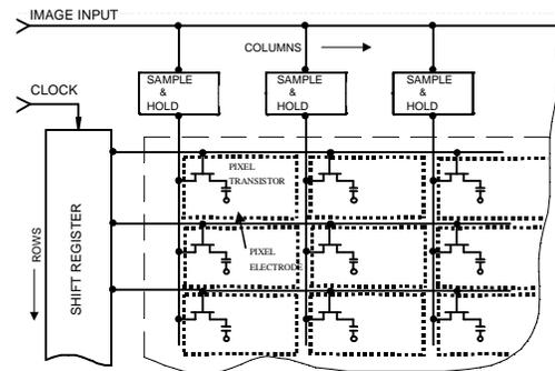
Fig. 3. Schematic of image information flow in the D-ILA device
